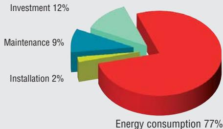
The diagram refers to a system with a 45 kW compressor, 5 year depreciation, 4000 hours/year, operating pressure 7 bar.
