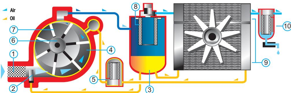
reduction of the spaces between the rotor-blades and the stator. The compressed air and oil mixture passes through various separating phases mechanical and coalescent, leaving less than 3 mg/m<sup>3</sup> in the air. The purified air leaves the compressor and is cooled in the radiator. The condensate which is produced is eliminated by a separator with an electronic condensate drain.
